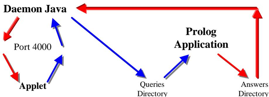
Figure 4: Scheme of the functioning of the MHITS Communicator Agent (Daemon Java)
