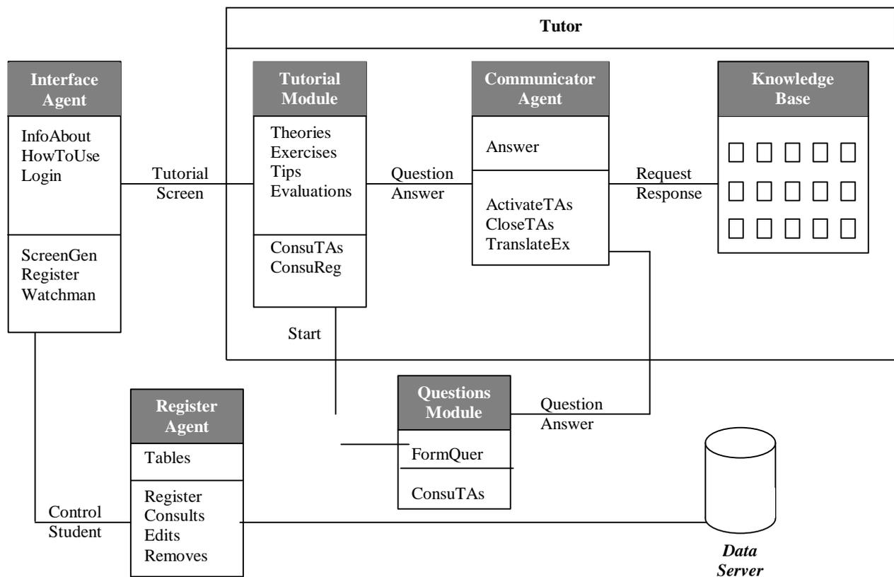
Figure 3: MHITS object diagram
