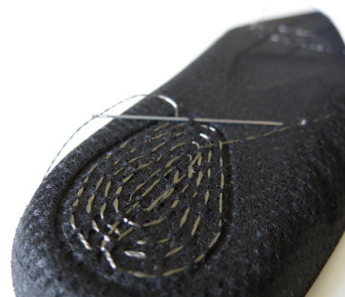
Figure 5: DIY sensor made out of a conductive foam insole and conductive thread electrodes
