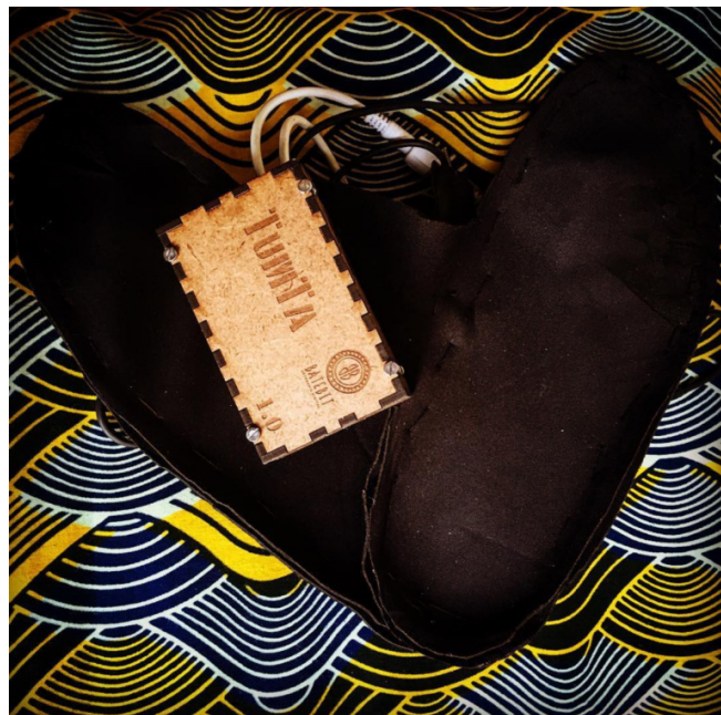
Figure 1: TumTá's insoles and transmitter hardware
