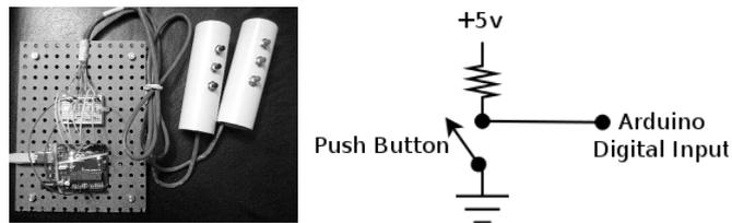
Fig. 2. The “Braille handle” device and pushbutton connection.
