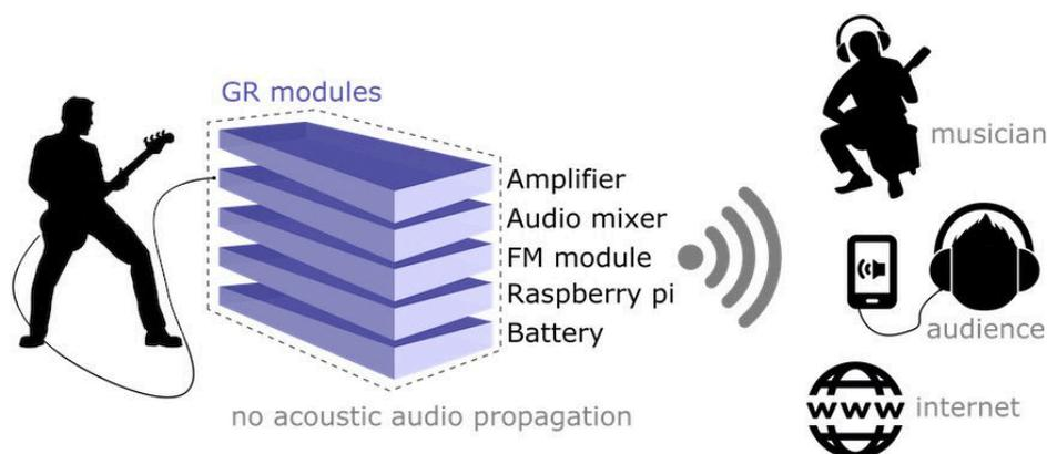
**Figure 1.** This figure shows the actual idea for the modular design of the next version of Gambiarradio, and how it works in a performance.
