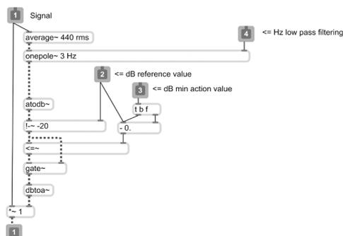
Figure 2. Adaptive signal level scaling, Max/MSP implementation
