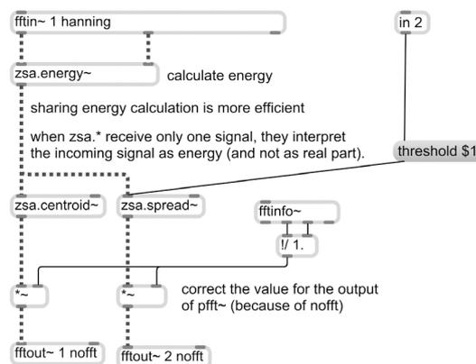
Figure 13. Patcher detail from *pfft~* object from Figure 12
