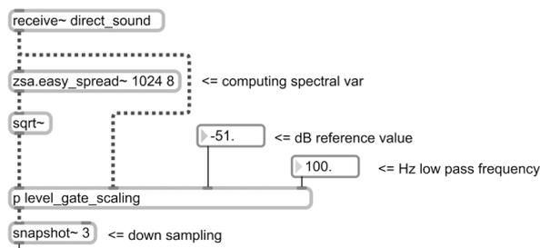
Figure 8. Gated spectral standard deviation, event detection function
