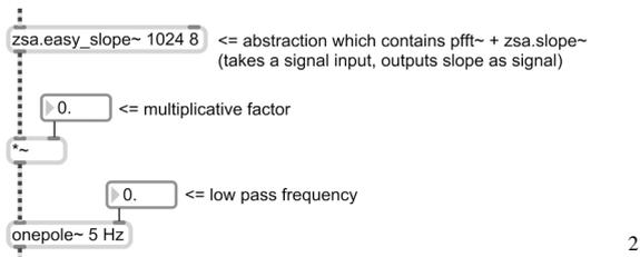
Figure 3. Spectral slope detection function
