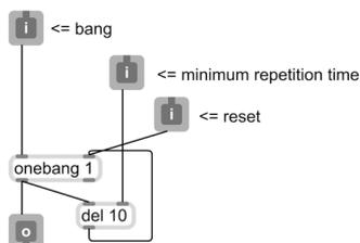
Figure 5. Delayed gate to avoid unwanted repetitions
