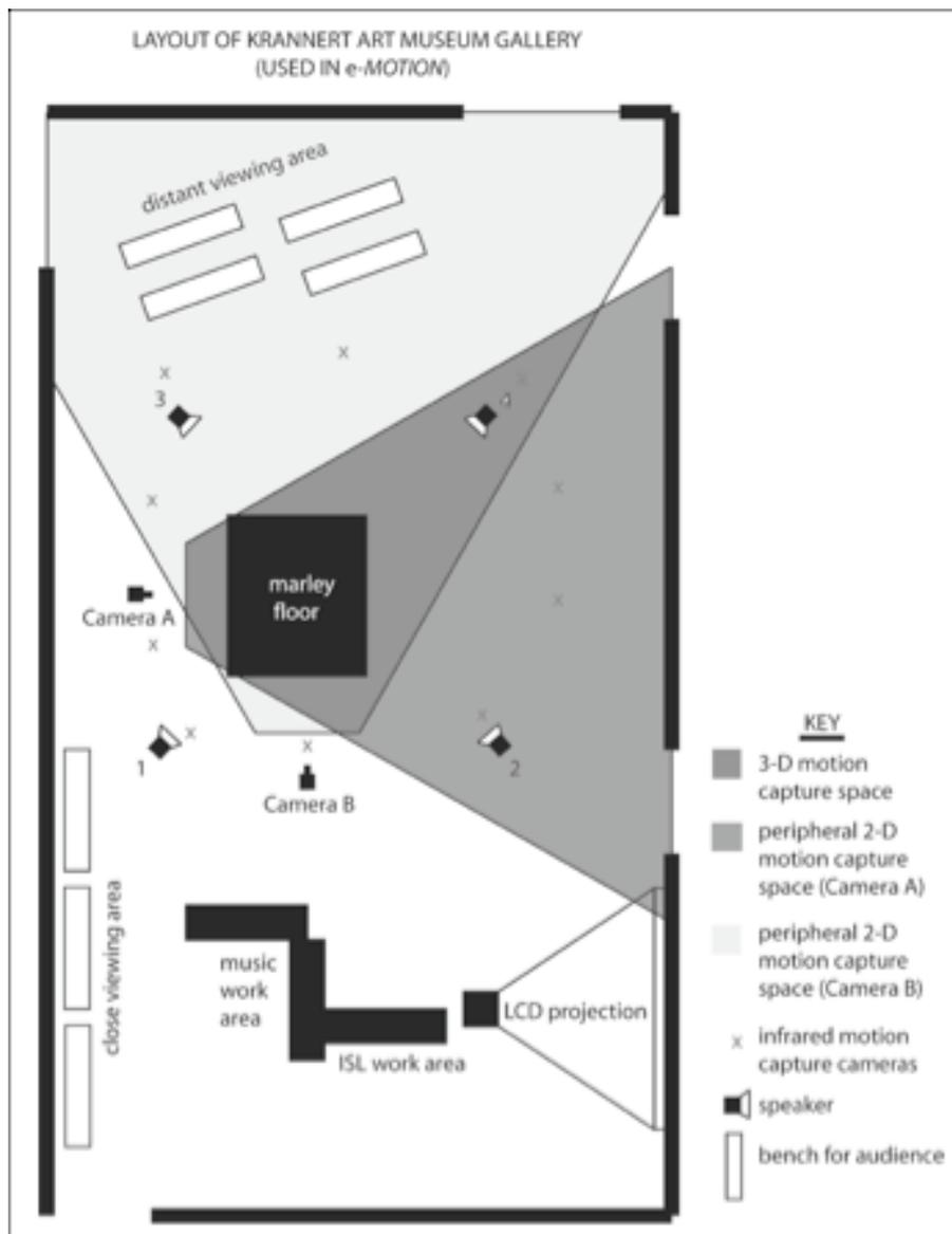
Figure 1. Camera arrangement
