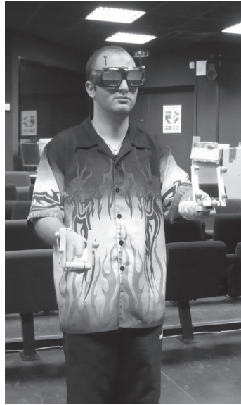
Figure 5: Using wii remotes with 6DOF tracking to control the virtual rays
