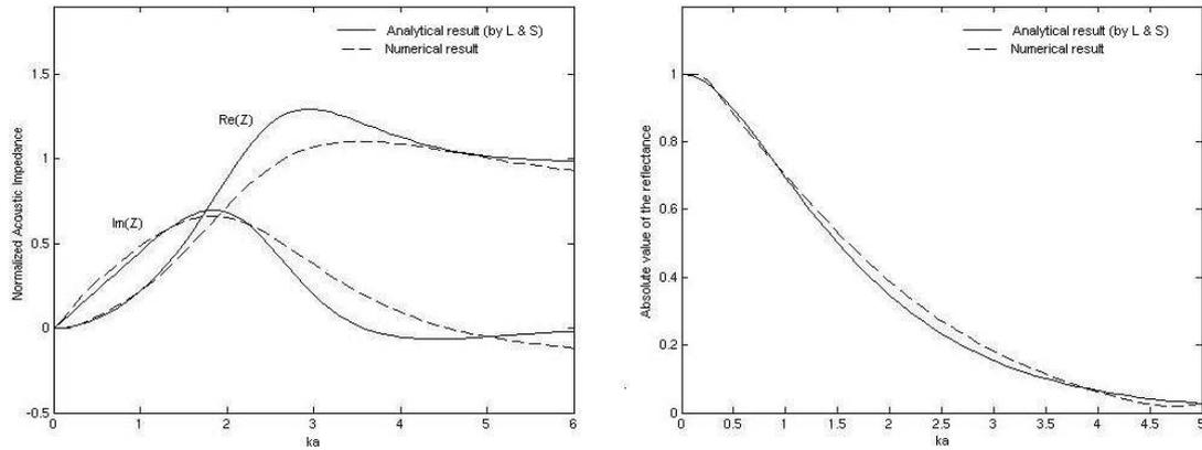
**Figure 2: Normalized impedance and reflectance as functions of  $ka$**
