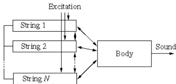
**Figure 3. Basic block model for a bowed string instrument. Depicting the excitation of more than one string.**
