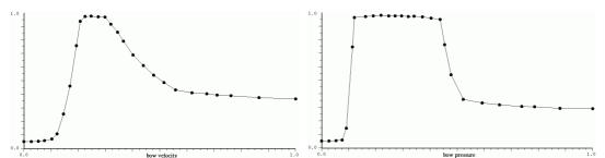
Figure 8. Envelopes of bow force and velocity in martelé (marcato) bowing style of one bowing period as function of time. The figure shows the general form of these parameters for physical modelling synthesis.
