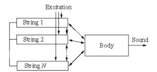
Figure 3. Basic block model for a bowed string instrument. Depicting the excitation of more than one string.
