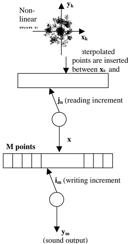
**Fig. 1** – FracWave structure diagram.
