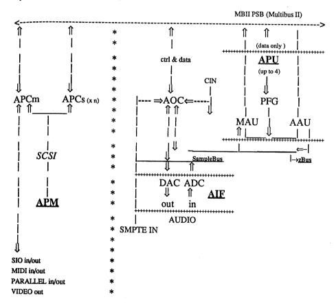
The hardware architecture of the AUDIAC has been concieved with the principle of the <u>specialized subsystems</u>. It has not only been made to generate organized forms for the musical production, but also incorporates the generation and working up of sounds in real-time. The whole implies a hughe measure of different demands in relation of its computing potential, which can only be solved with the above mentioned subsystems and their communication capacities.
